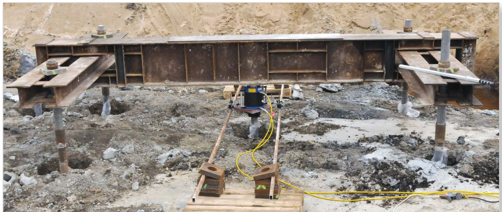
Compression loading test on micropiles in soil with a risk of buckling.
