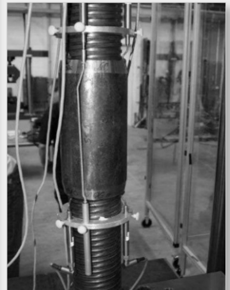
Fatigue test on TITAN 103/78 coupler connection at TU München
