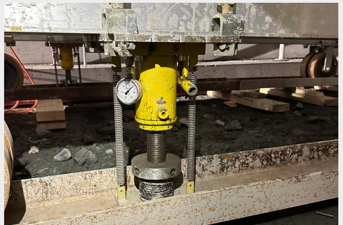
Hydraulic cylinder to disengage the wheels
